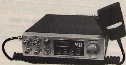
PRESIDENT MOD. JACKSON 227 canali AM-FM-USB-MSB II - 40 - 45 m 10 W in AM - 21 W SSB
